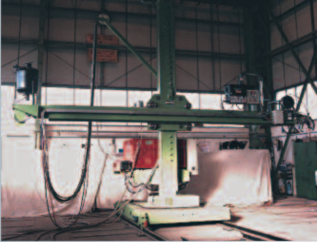
Model 3/TRMB 4 m x 5 m Tracked unit with rotating column.
