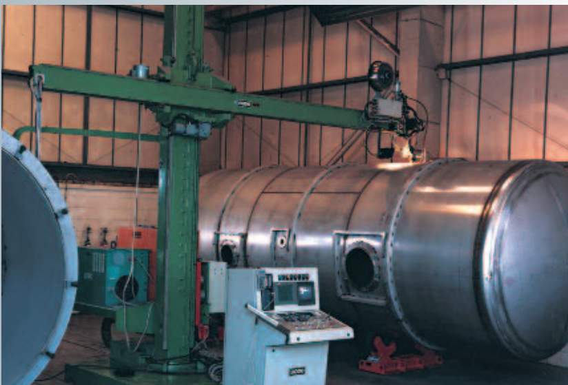
Model 3/TRMB Utilised as shown in stainless steel container welding role. Container carried on Bode SAR 1200 Rotators. Remote control master station.
