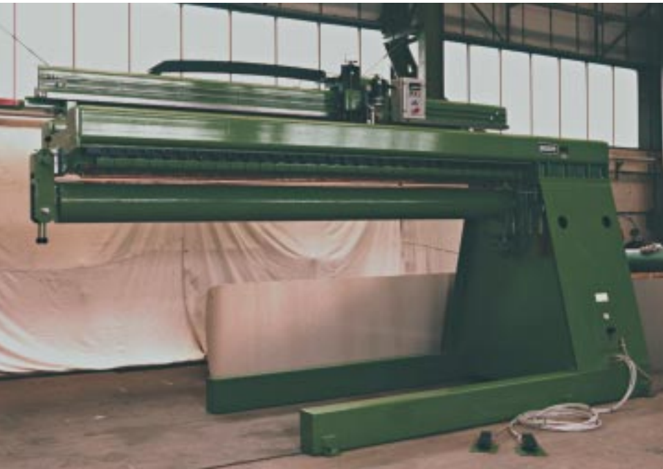
9/HSW 2500 - 3000 Special model with manual elevation of the mandrel
