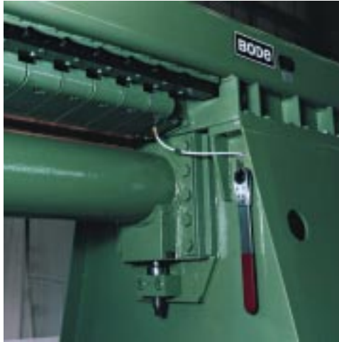
9/HSW 2500 - 3000 Special model with manual elevation of the mandrel
