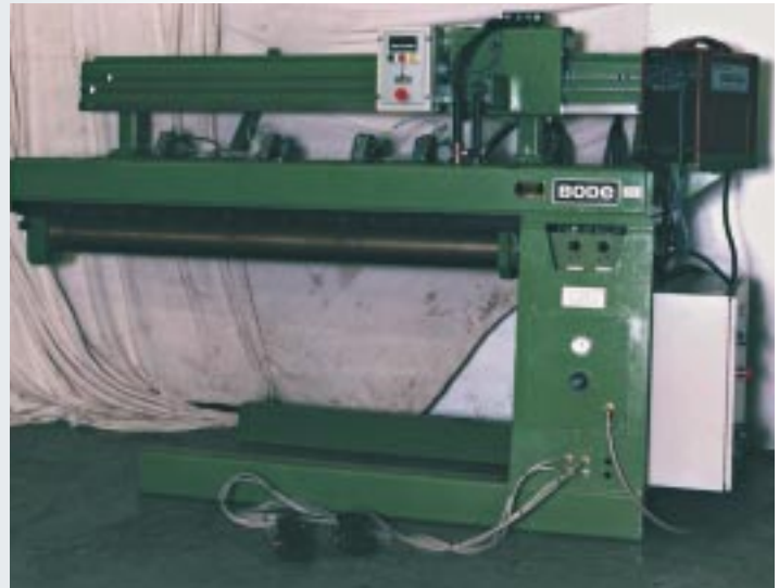
5 HSW 150-1600 5 HSW 150-1600 seam welder fitted with Tig welding equipment. Max clamping length 1600 mm Max diameter of workpiece 800 mm Min diameter of workpiece 150 mm
